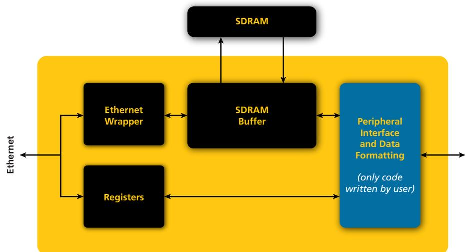
Figure 2: Arrangement of cores in a ZestET2 Ethernet board
