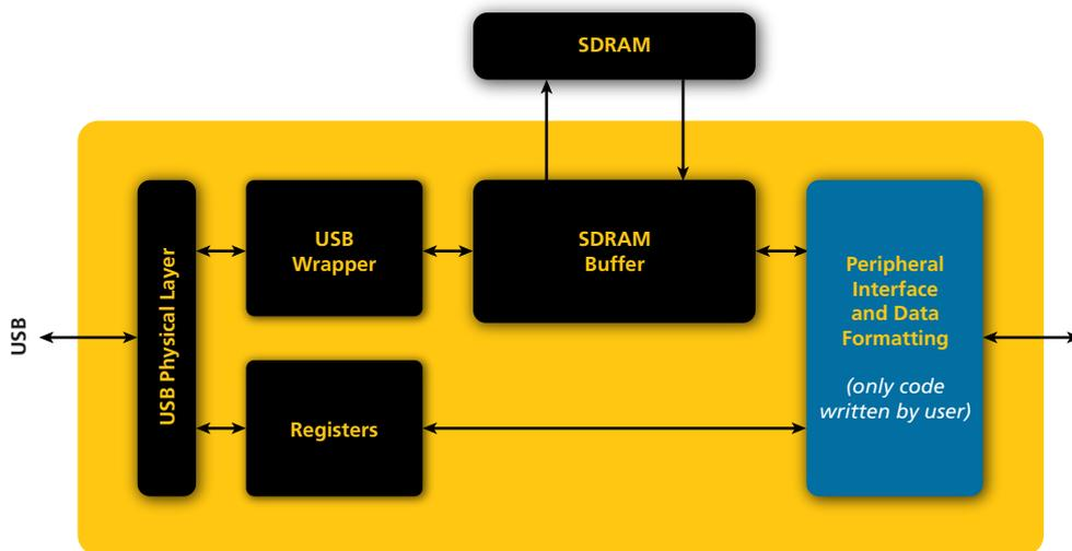
Figure 3: Arrangement of cores in a ZestSC3 USB board
